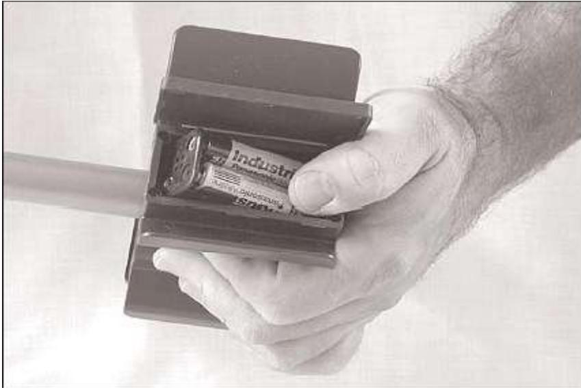
When returning the holder, note the position of the spring clips inside the armrest housing and make sure that the battery pack contacts fit snugly against the springs. Insert the side with the contacts first and then press down on the left edge of the battery holder to reseal the holder.
