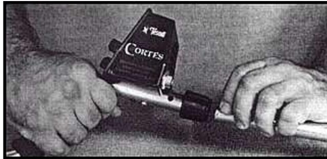
6. Slide lower pole into middle pole until the spring buttons click into the first set of adjustment holes. Turn pole lock to tighten, thus locking the assembly into place.
