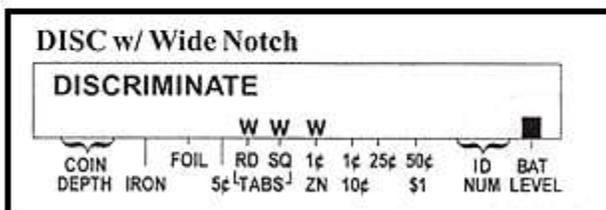
These indications are an easy way to check what part of the scale is being notched out. The notch indicators will only show when there is no target under the coil. When there is a target signal, no matter if the target has been discriminated or not, the display will show the information of the target. Take some time to try various targets and note the response. When you are done, flip the NOTCH switch back into the center position before moving to the next section of the quick start.
