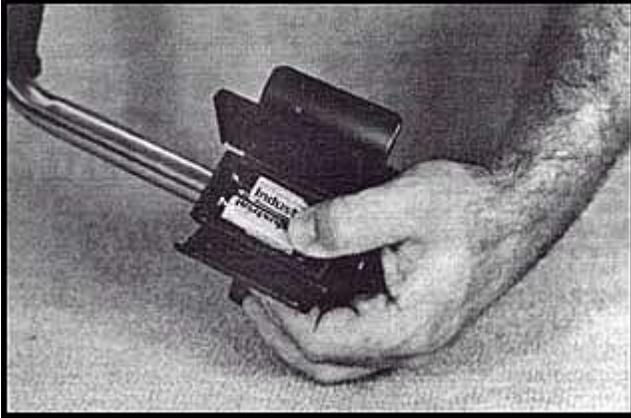
Remove the batteries by pressing down on the right side of the 4-pack battery holder so that the left side of the holder will pop up. Pull out the holder and replace the batteries as needed.
