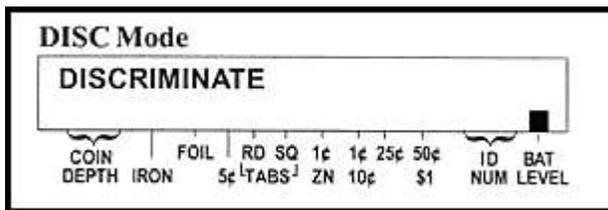
Pass any target over the coil and read the meter. The information is unimportant at this moment. After about 6 to 10 seconds the screen will clear and the word DISCRIMINATE will appear again. The Cortés will clear the display screen after that amount of time so you will be able to visually see a target even if you do not get an audio response. You may want to take some time to try this out.
