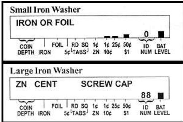
The thing that both of these illustrations have in common is that the various segments of the display do not "agree" with each other. This is a sure sign that you are detecting an odd-shaped piece of iron. Notice on the rest of the illustrations that the bar graph and the ID number show about the same information. When the ID number and the graph "agree," you can be sure that your Cortés is receiving a clean signal.
