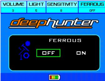
If the user desires, the device can be adjusted to eliminate ferrous metals and not report them to the user. To use this feature the FERROUS setting must be disabled.
