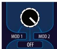
Turn the On/Off button to the Mode 2 position. When the device is turned on, the opening sound will play. After approximately 10 seconds, the device will be ready to use with the active audio alert.
