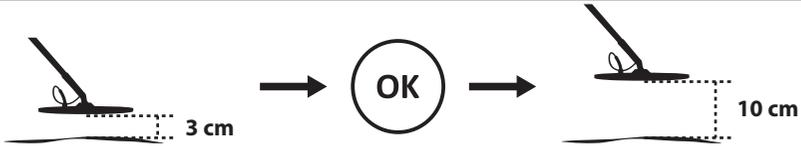
After the effect is completely removed, press the OK button as the coil is lowered down to 10 cm. Now switch to the search mode and start searching.
