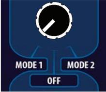
The device has two separate systems. These systems are called Mode 1 and Mode 2. Turn On/Off button to "Mode 1" position to operate the device with the screen system. Mode 1 is the operating mode in which the data obtained is presented to user with views and sounds. This mode is used for detection of larger targets at significant depth.
