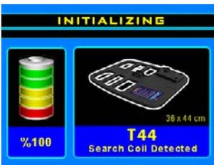
The Device automatically identifies the coil which is attached to it at the time when it is turned On. The coil attached will be shown on the screen. If a coil other than the appropriate one(s) is attached to the device, this will be indicated on the screen as "COIL FAILURE" warning. In addition, data regarding the battery status is also shown on the same screen.
