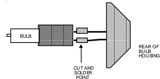
**CAUTION:** The bulbs should not be handled with bare fingers as oil from the skin gets onto the glass and will cause the bulb to burn up. If the bulb is handled with bare fingers, the glass should be wiped with denatured alcohol to remove any oil from the glass.
