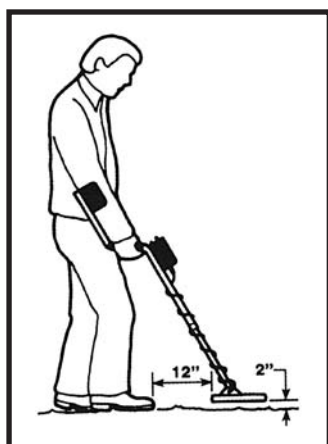
Figure 2. SEARCH POSITION. Adjust the stem length and coil angle so the coil rests flat on the ground about 6 to 12 inches in front of your foot. Move into your "search" position by leaning forward slightly and raising the coil about 2 inches off the ground. This should put the search coil out about 12 to 18 inches in front of your foot.
